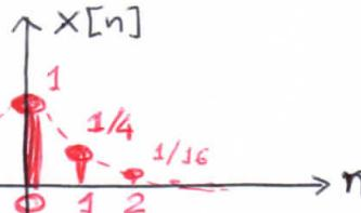
$$P_{2N+1} = \sum_{n=-N}^N |x[n]|^2 = \frac{1}{2N+1} \left( \lfloor \frac{N}{2} \rfloor + \sum_{n=0}^{\lfloor N/2 \rfloor} \left( \frac{1}{16} \right)^n \right)$$
